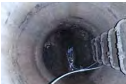
Sampler intake teflon tubing, strainer pointing downstream
