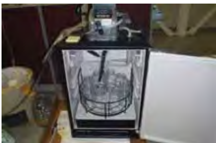
Automatic sampler with eight sample bottles
