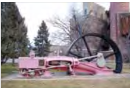
James Watt’s centrifugal governor on “Old Sally,” a 150-Hp steam engine installed in 1881 at Boulder, Co. A shot of steam drives the balls (top, center of photo). As the balls spin faster, they stand out by centrifugal force and levers raise a valve stem that opens to relieve excess pressure and governs the engine’s velocity. This mechanical device is the history of instrumentation.
