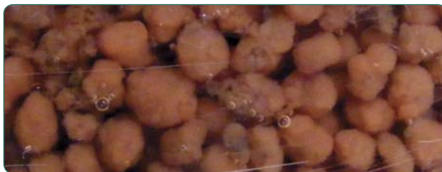
Figure 1: Shows anammox flocs in an ongoing reactor fed with real filtrate.
