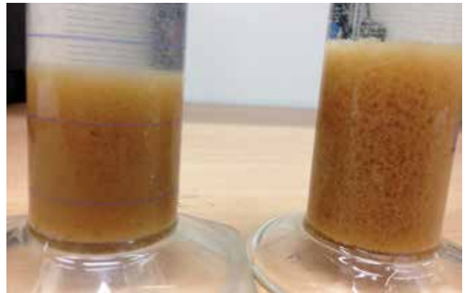
Fig 1. (b) Conventional reactor biomass (left) and Granular reactor biomass (right).
