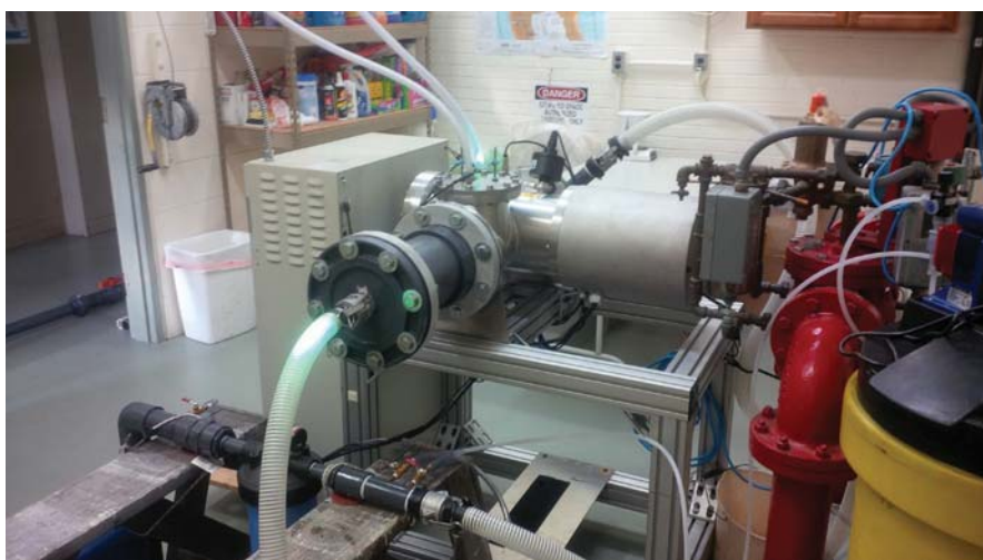
Picture of ETS AOP pilot system that uses an advanced electrode to generate trace amounts of OH - and ClO - / HOCl in situ from typical levels of TDS in the raw water. The active species are formed immediately upstream of the UV lamps, and effectively consumed during the AOP process.
