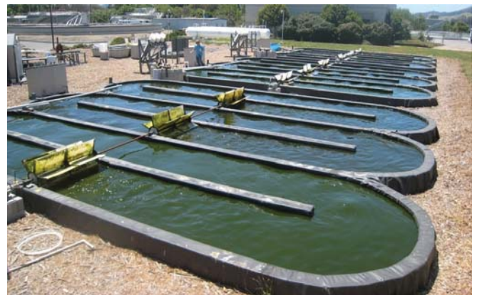
Figure 2. Raceway Algae high rate pond. Credit: Lundquist, T., Spierling, R., Parker, L., Pittner, C., Medina, L., Steffen, T., Alvarez, J., Adler, N., and Benemann, J. (2016). "The RNEW® Process: Recycled Water, Fertilizer, and Power from Wastewater," presented at Algae Biomass Summit, Oct. 23, 2016, Phoenix, Ariz.
