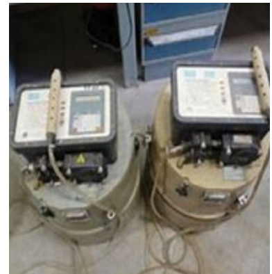
Automatic samplers can collect composite samples according to a time schedule or metered flow.
