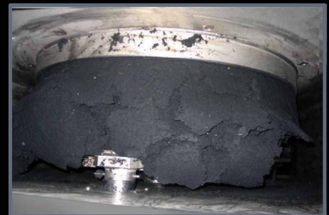
Dewatered Anaerobic Biosolids
