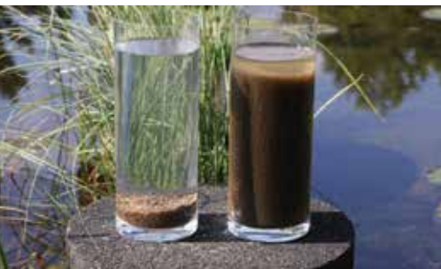
SVI 5 comparison of aerobic granular sludge (left) and conventional activated sludge (right)
